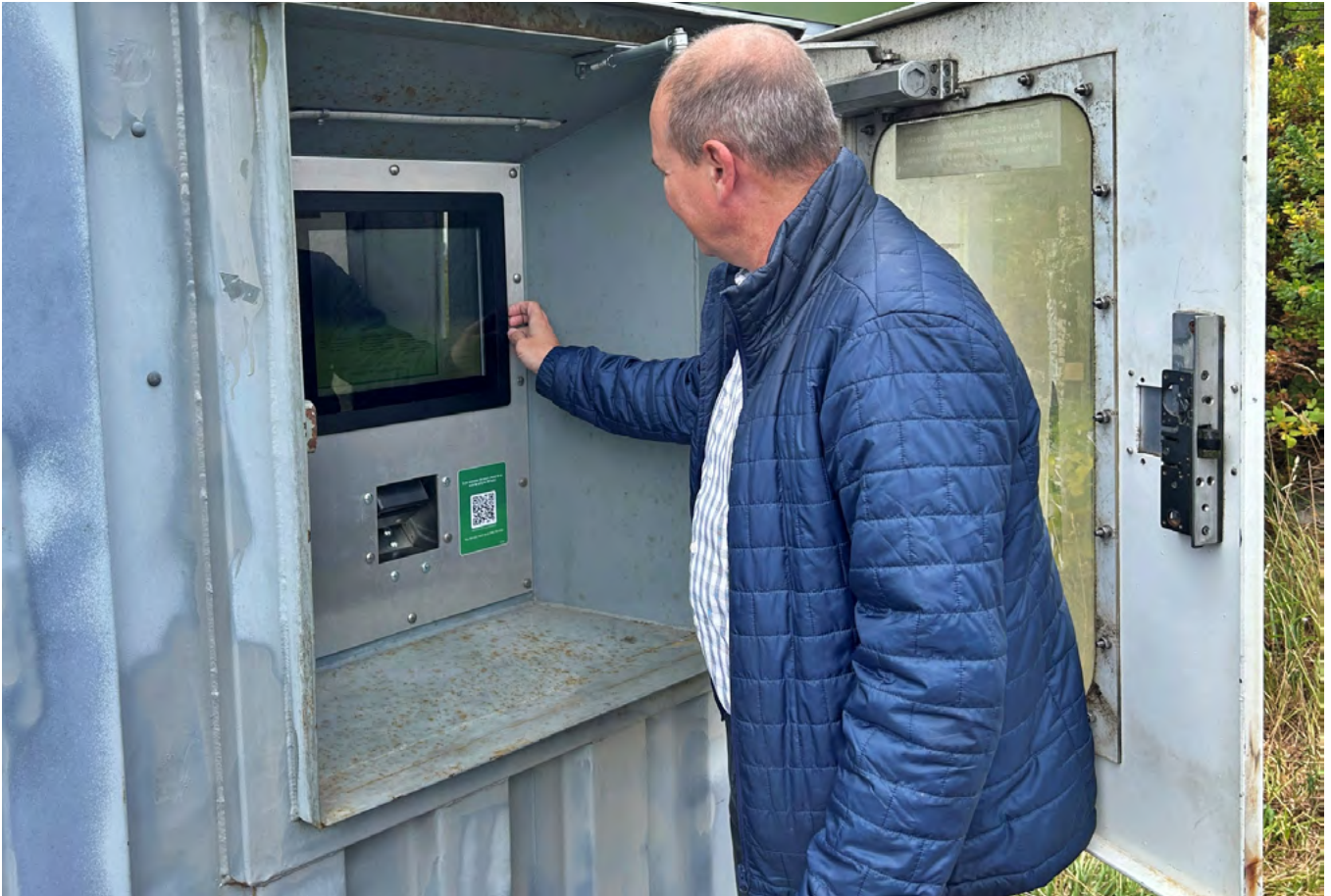
Mike Wadden demonstrates the use of an Xpress screen (this one on an outside UCycle). This allows customers to print bar-coded tags and drop off their recyclables, which will be counted later and credited to their account. Photo: L. Vryenhoek
