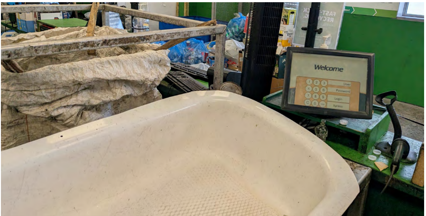
At stations in the facility, workers receive beverage containers from customers. They dump the containers into repurposed bathtubs for sorting, and operate a touchscreen to record what the customers have dropped off. Photo courtesy of Ever Green Recycling.
