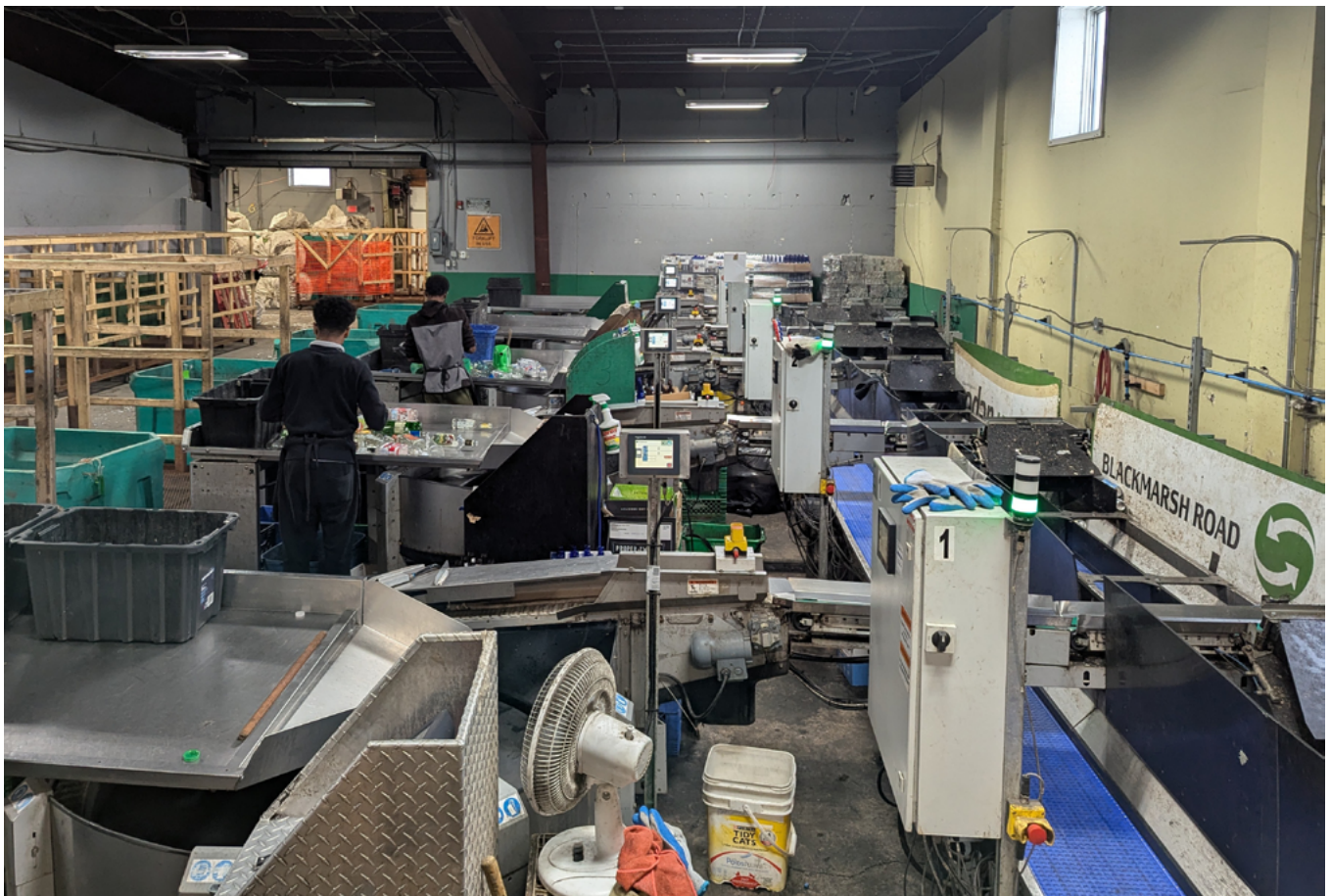
Ever Green workers sort cans and bottles in the back of house area of the Blackmarsh facility, where a system of conveyor belts helps with processing. Photo courtesy of Ever Green Recycling.
